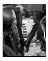
9. Connect the other end of the negative (-) cable to the remote negative (-) terminal, marked GND, on the vehicle with the dead battery.
